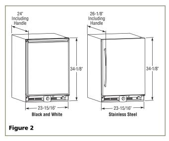
Please note that the unit has adjustable feet that can add one additional inch to height during leveling or to match adjacent cabinets (see **Figure 43** on **Page 17**).
